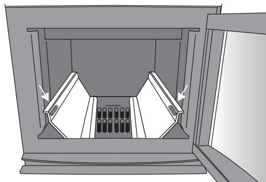
**Figure 2. Combustion air channels**
