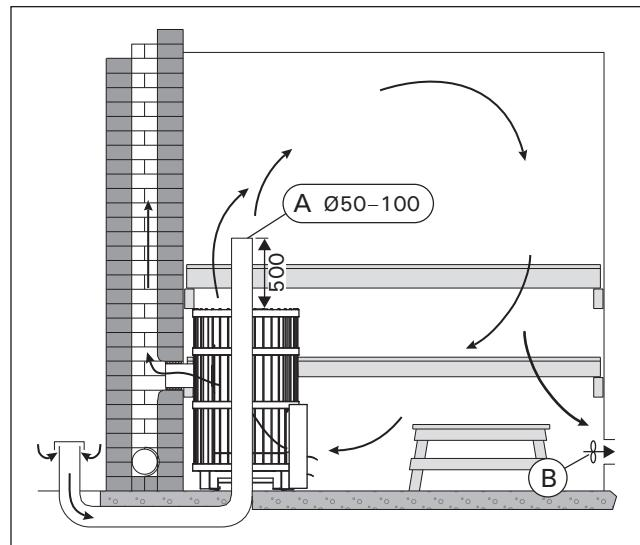
Figure 7. Mechanical exhaust ventilation
