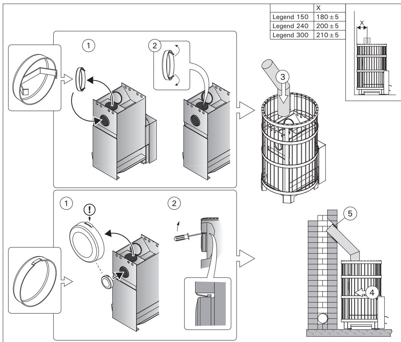
Figure 12. Connecting the stove to a masonry flue via the upper connection opening (all dimensions in millimeters)
