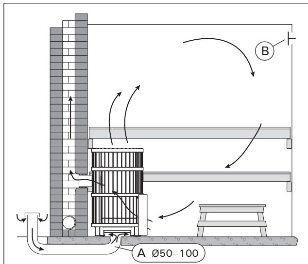
Figure 6. Gravity exhaust ventilation
