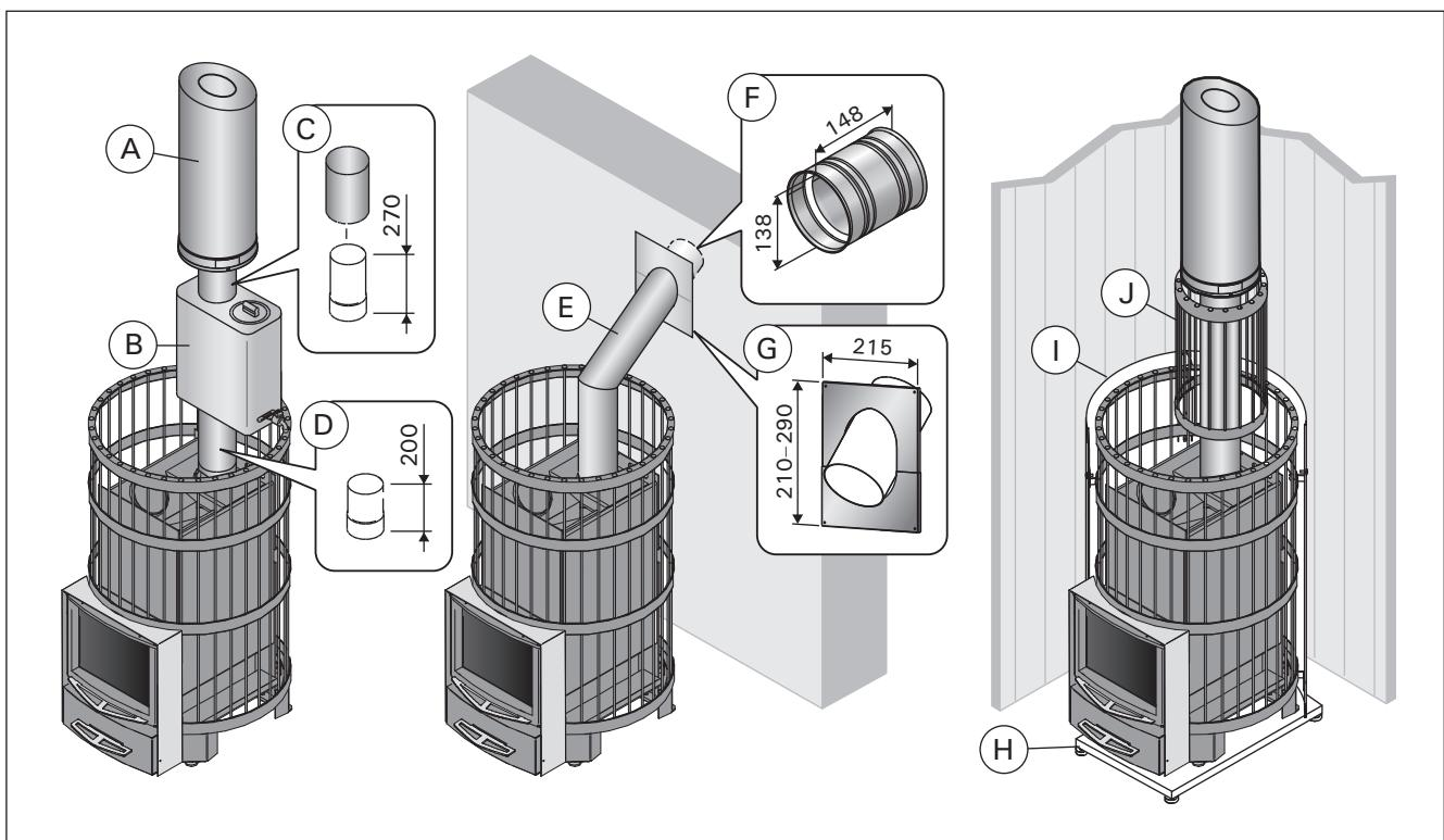
**Figure 17. Accessories (all dimensions in millimeters)**
