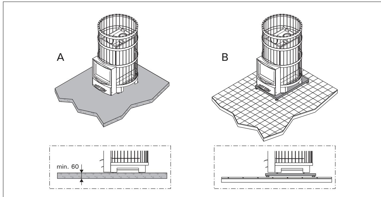
Figure 8. Protecting the floor (all dimensions in millimeters)
