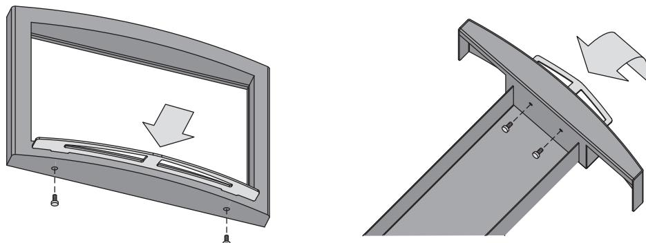
*Figure 16. Installing the handles
