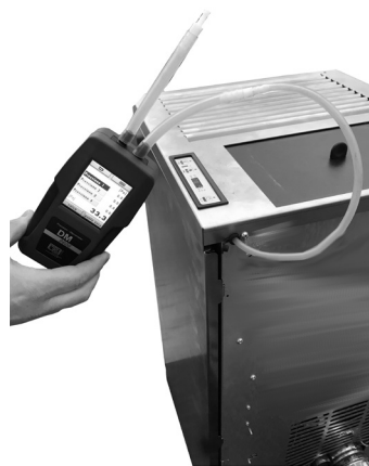
Fig. 53 - Digital pressure switch connection
