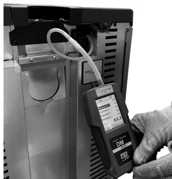
Fig. 51 - Digital pressure switch connection
