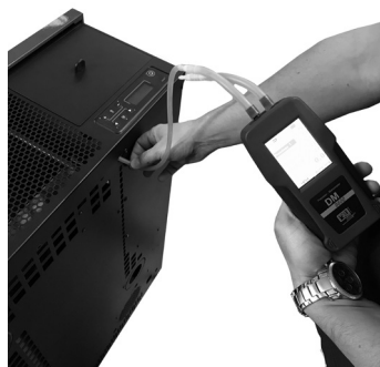
Fig. 39 - Digital pressure switch connection
