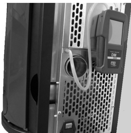
Fig. 50 - Digital pressure switch connection
