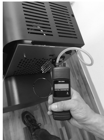
Fig. 49 - Digital pressure switch connection
