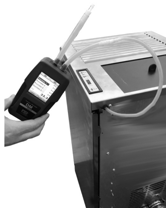
Fig. 55 - Digital pressure switch connection
