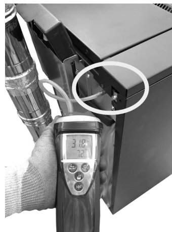
Fig. 43 - Digital pressure switch connection
