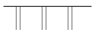
Firewall, approved and fully complies with safety requirements according to the authorised inspection body. Examples of approved firewalls are 120 mm solid brick and 100 mm aerated concrete.
